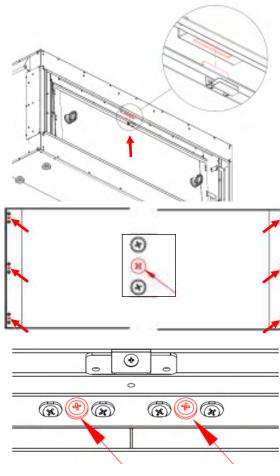
Trim Installation **3.5.2** Once the non-combustible board has been fixed to the studding, the trim can now be fitted to complete the installation.
