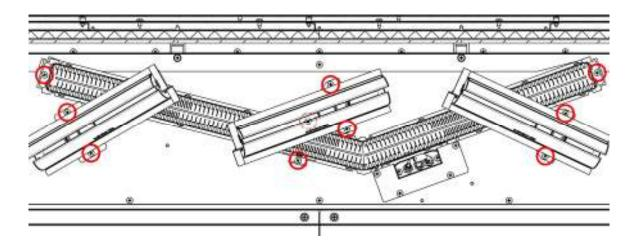
The main burner injectors can now be seen and can be removed with a 7mm box spanner.
